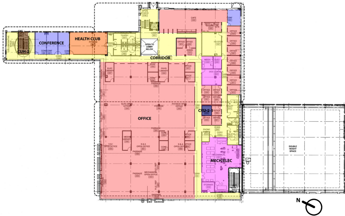
Figure 1-2-2: Second Floor Zones (AHU-2).
