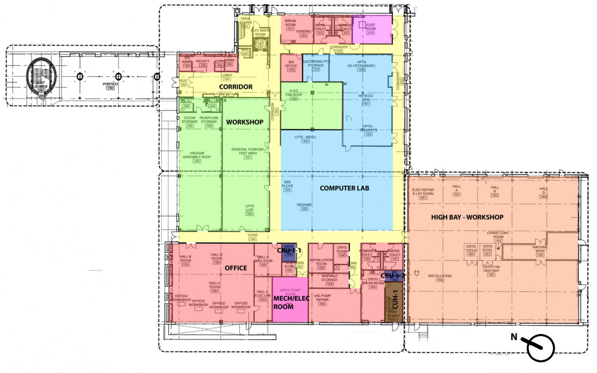
Figure 1-2-1: First Floor Zones (AHU-1).
